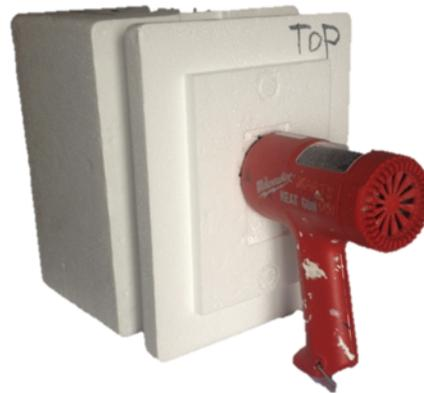
To stop heat from escaping around the sides we acquired a Styrofoam cooler (courtesy of Jeffrey Oda, USF Dept of Biology). A 7"x7.5" rectangle, 0.5" deep, on the outer side was cut out for a piece of bark to be placed while heating. Then a 2"x2" square was cut out on the other side for the heat to transfer through the bark. This minimized heat escaping around the edges.
